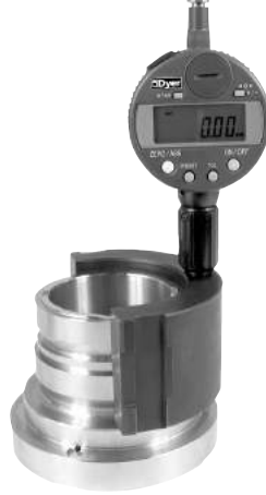
Outside shoulder/groove height. Measure bottom surface of part to top of groove.
