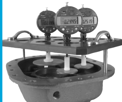
Special fixture to measure multiple bore depths at one time on a machined casting
