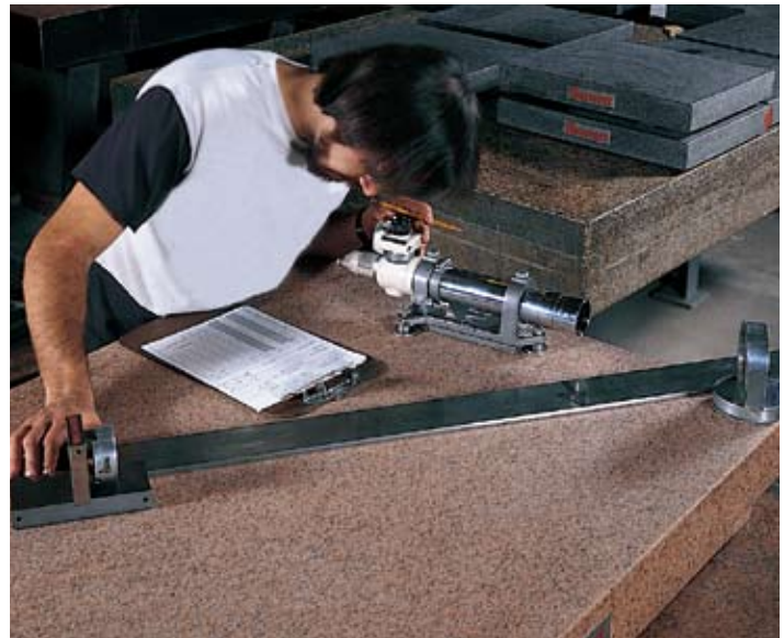
Inspecting a granite plate with an autocollimator.
